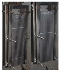
*Fig. 1. Ignitability test (flame application to surface and bottom edge).*
